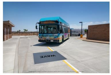
With power ranging from 125kW to 500kW and higher, WAVE's high-power systems deliver fast, safe, high-power charging within seconds of scheduled stops and natural dwell times.
