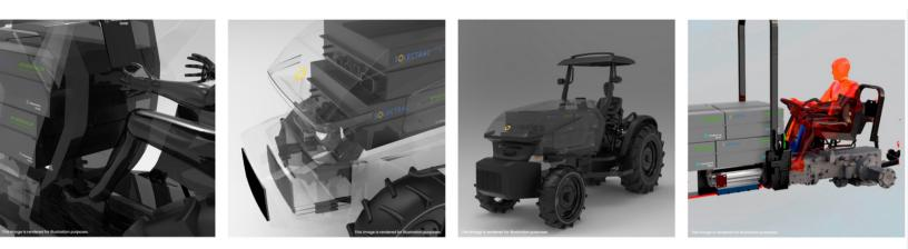
Guided by Ideanomics Design's vision for the e75N's design, Energica Inside is leading the development, assembly, testing and validation for the tractor, an end-to-end process that starts from the CAD drawing and reaches a validated prototype.
